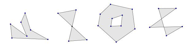
**Definition 3.** A polygon P is called **convex** if given any two points x, y inside the polygon, the line  $\overline{xy}$  is contained entirely inside of P. Otherwise, the polygon is called **nonconvex** or **concave**.
