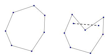
Figure 1: A convex polygon (left) and a nonconvex polygon (right)
